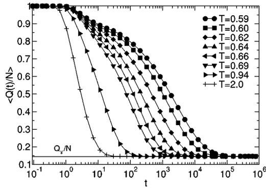
FIG. 3. Average time-dependent overlap “order parameter”  $\langle Q(t)/N \rangle$  for each state point simulated. The solid line corresponds to the random value  $Q_\infty/N=0.147$ , as discussed in the previous section.
