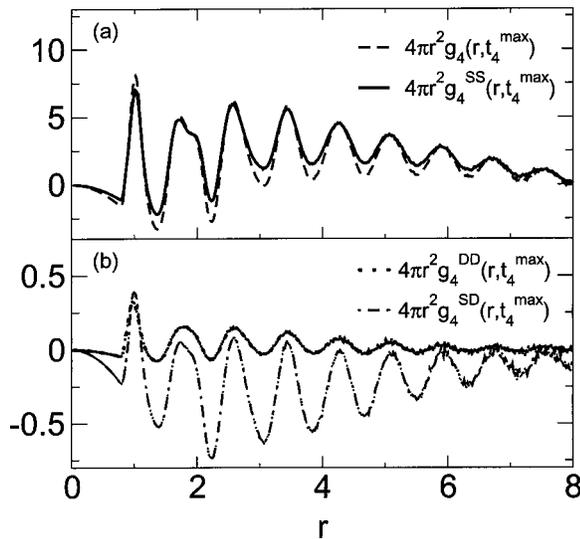
FIG. 16. (a)  $g_4^{SS}(r, t_4^{\max})$  (solid line) at  $T=0.62$ . The dashed line shows  $g_4(r, t)$  for comparison. (b) Distinct (dotted line), and self-distinct (dot-dashed line) parts of  $g_4(r, t_4^{\max})$  at  $T=0.62$ . We separate the contributions into two panels due to the large difference in amplitude.
