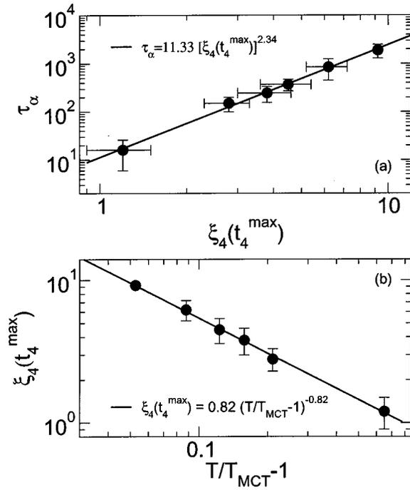
FIG. 14. (a) Log–log plot of  $\tau_\alpha$  vs  $\xi_4(t_4^{\max})$ . (b) Log–log plot of  $\xi_4(t_4^{\max})$  vs  $T/T_{\text{MCT}} - 1$ . Solid lines are power law fits using equations similar to Eq. (2).
