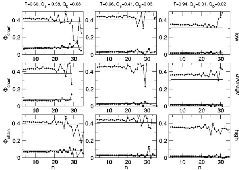
**Figure 14.** Fraction,  $\Phi_{\text{chain}}$ , of localized and replaced particles for low, average, and high force chains. The fraction of localized and replaced particles at  $t_4^{\text{max}}$  is marked with the corresponding  $T$ , and it is indicated by the solid lines on each panel.
