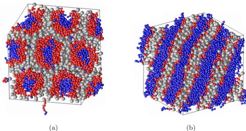
Fig. 6. Simulation snapshots of diblock copolymer tethered nanosphere morphologies. (a) Core-shell cylinders are observed in selective good solvent at  $f_B = 0.75$ . (b) Lamellae in an ABCCBA pattern are observed in neutral poor solvent at  $f_B = 0.25$ .
