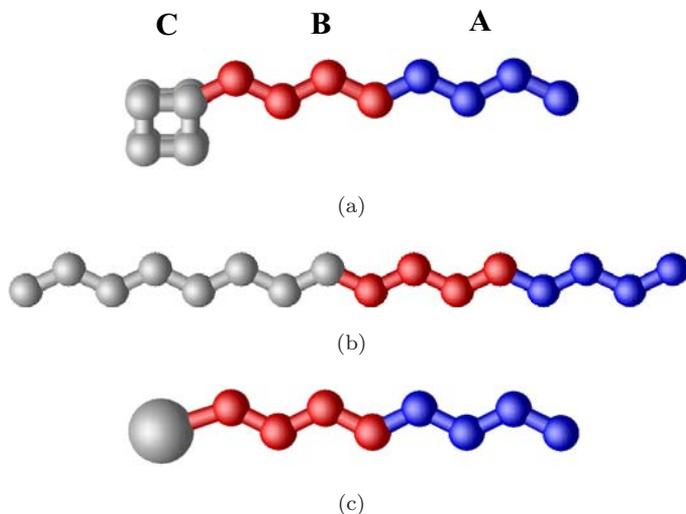
Fig. 2. Representations of model monotethered NBBs with a diblock copolymer tether attached to either a nanoparticle or its linear chain counterpart. (a) ABC diblock copolymer tethered nanocube. (b) Linear ABC triblock copolymer. (c) ABC diblock copolymer tethered nanosphere.
