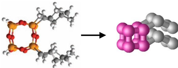
Fig. 1. Representation of a tetrasubstituted POSS molecule  $\text{R}'_4\text{R}_4\text{Si}_8\text{O}_{12}$  (left) by the minimal model (right). There are four homopolymer tethers  $\text{R}'$  each attached to silicon atoms that comprise the same face of the cubic cage. In the atomistic representation, the silicon atoms are denoted in orange, carbon atoms in grey, oxygen atoms in red, and hydrogen atoms in white.
