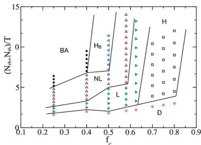
Fig. 2 Morphological phase diagram for low aspect ratio tethered rods. Black circles, upward pointing maroon triangles, left pointing blue triangles, right pointing green triangles, and black squares denote the bilayer arrowhead (BA), nematic lamellar (NL), hexatic B ( $H_B$ ), lamellar (L), and hexagonal cylinder morphologies (H), respectively. The red diamonds denote the disordered state (D).
