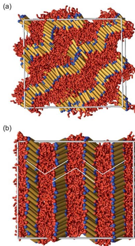
**Fig. 12** Simulation snapshot of (a) the wavy lamellar morphology and (b) simulation snapshot of the interdigitated arrowhead morphology. The white lines denote the v-shaped patterns formed by neighboring rod layers.
